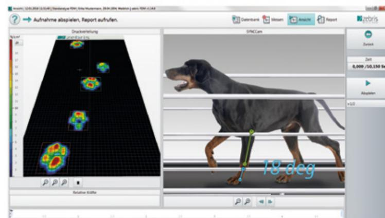
The roll-off details of the animal are presented in slow motion, whereby the joint angle of limbs can be measured directly on a display screen.
