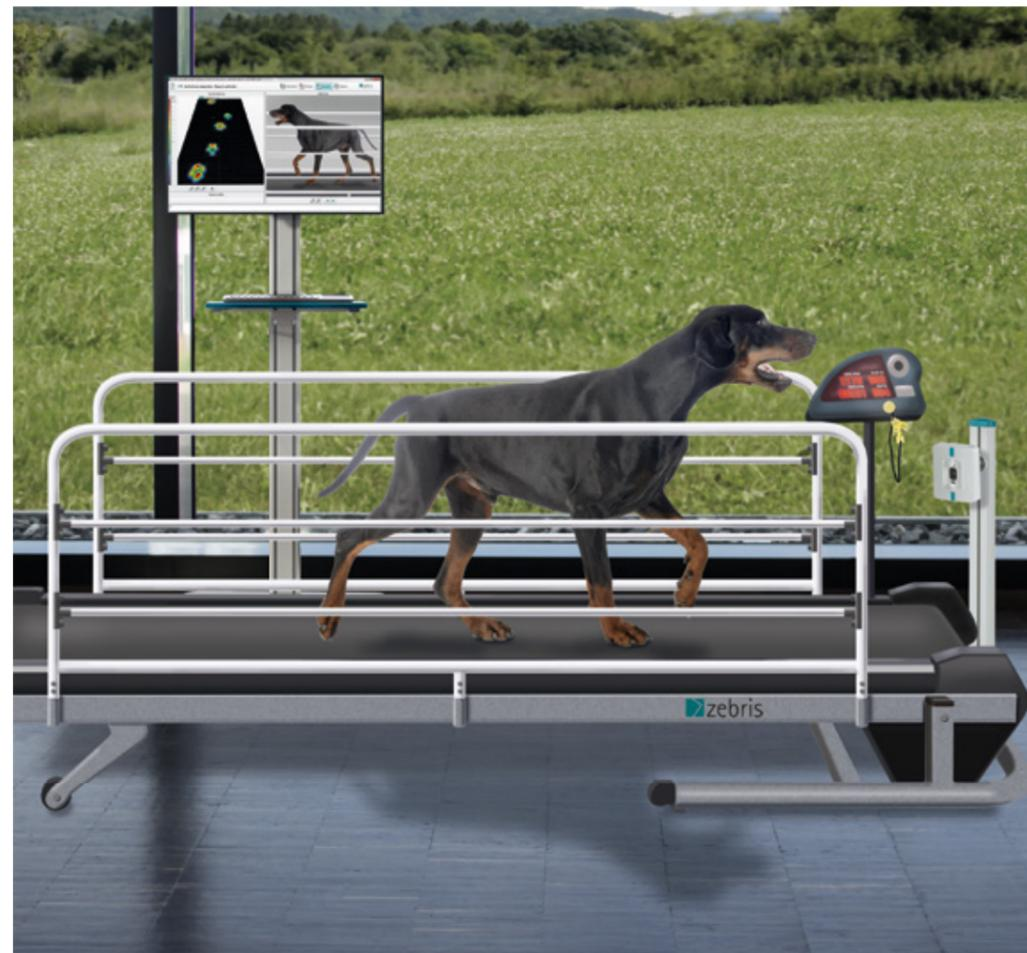
The system consists of a treadmill or platform equipped with a calibrated pressure sensor matrix and one or several synchronised cameras.
