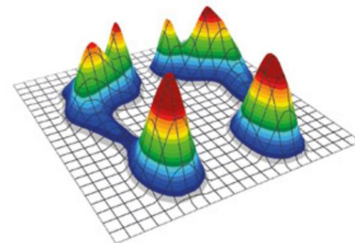
The pressure measurement plate contains high-quality capacitive sensors for precise determination of balance and movement quality
