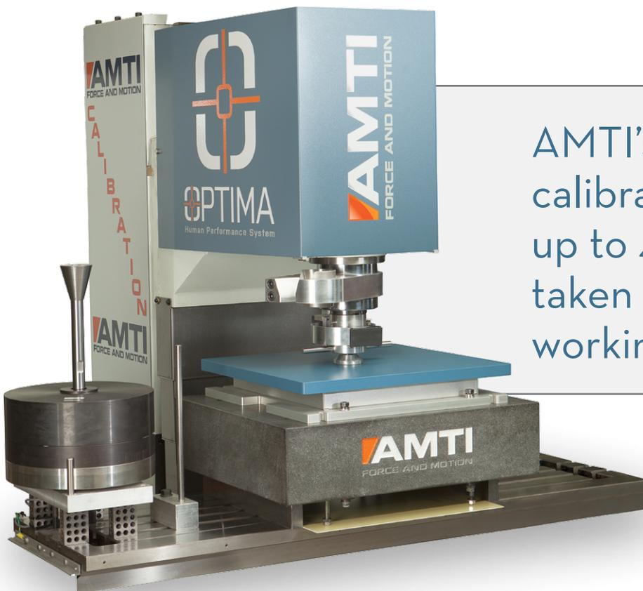
AMTI's patented OPTIMA calibration process involves up to 4000 measurements taken over the entire working surface of the plate.
