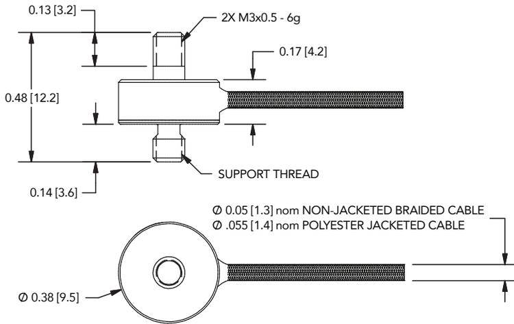
Note: Static one time bends are not to exceed 2-3 times the diameter of the cable. Continuous bends should not exceed a radius of 10 times the diameter of the sensor cable. Polyester Cable versions are available to offer support for applications with cable movement.
